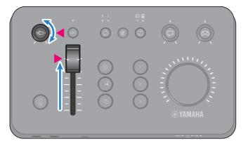
You can use Yamaha ZG Controller to check the mic input/output levels. Adjust the input level (MIC LEVEL) and output level (OUT LEVEL) while checking the level meters on the "MIC SETTINGS" screen, so that the levels are within the "OK" range.
