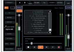
Media player with simultaneous recording Play multiple formats from MP3 to WAV ONE TOUCH OPERATION TO PLAY (records L/R main mix in stereo WAV)
