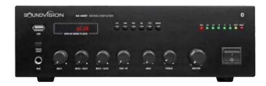
**The SA-60BT** USB/BT Portable Mixing Amplifier Compact provides 60 watts of output power with Bluetooth, integral USB audio player power, and 5 inputs including 3 balanced MIC (MIC1 has another port of 6.35mm jack on front panel), 2 unbalanced AUX, each one has individual volume control.
