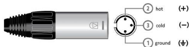
MIC INPUT Balanced male XLR
