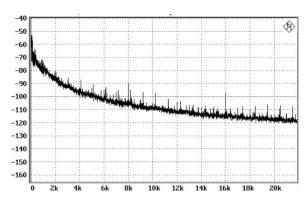
We can see that the noise floor at 1kHz is about -75dB and at 10kHz it is about -110dB.
