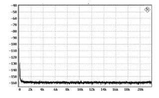
The results are limited by the capabilities of the measuring equipment and noise floor lays at –160dB or even lower. There are visible peaks at 50Hz and 100Hz which are caused by limits of the measuring instruments. However, they are at a level of –130dB and –140dB.
