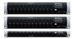
**StudioLive Series III rack mixer.** The StudioLive 16R, 24R, or 32R can be used to convert up to 32 channels of analog sources to digital audio that can be sent to EarMix 16M personal monitor mixers over the AVB network. More than just input modules for analog-to-digital conversion, these mixer provide noise gate, compressor, EQ, and limiter on every input channel, plus flexible mix buses to simplifies larger mixes, reverb, and delay.
