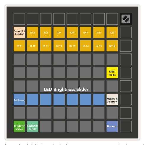
The **LED brightness level slider** has 8 levels, from minimum to maximum brightness. The brightly lit white pad indicates which level is currently selected.
