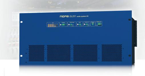
DL251 is a 5U 19" fixed-configuration rack I/O unit with 48 mic/line level inputs and 16 line level outputs and delivers legendary MIDAS sound quality utilising our time-tested and road-proven technologies. Featuring award-winning MIDAS microphone preamplifiers with 2.5 dB analogue gain steps and three AES50 network ports providing N+1 redundancy, plus an Ethernet control port and a MIDI Interface (In, Out, Thru), the DL251 is
