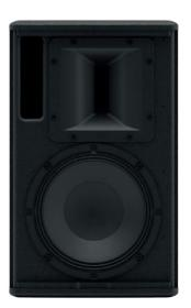
The X8 is an ultra-compact passive two-way system with an 8" (200 mm)/2" (50 mm) voice coil LF driver and a 1" (25 mm) HF driver mounted on a 90° x 50° horn which can be easily rotated for horizontal or vertical orientation, depending on venue requirements. Its very small size gives no indication of its high output capability.
