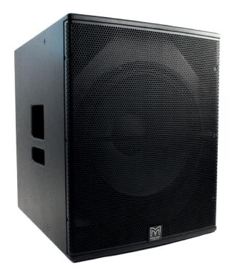
The X118 is a compact, high performance subwoofer for use with BlacklineX Series full-range loudspeakers. It extends the low frequency operating range of the combined system to 42Hz and provides exceptional low frequency impact. It can be used singly, stacked or flown via integral M10 insets and features a long-excursion 18" (460mm)/4" (100mm) voice coil driver in a compact reflex enclosure. Its four reflex ports have a large frontal area to reduce turbulent air noise at very high levels.
