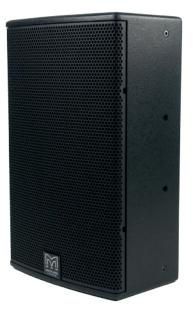
The X10 is a high performance yet very compact two-way passive loudspeaker system which utilises a 10" (250 mm)/2.5" (63 mm) voice coil LF driver and a 1" (25 mm) exit HF compression driver with a 1.4" (35 mm) polyimide diaphragm. The rotatable  $90° \times 50°$  HF horn has equal horizontal and vertical mouth dimensions for directivity control in both planes.
