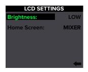
The parameter on top is LCD brightness. Push the speaker control knob again to edit the brightness. There are three choices: low, high and off.
