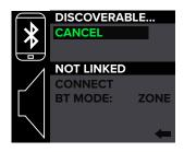
(3) The text "discoverable..." will change to "paired" and "cancel" will change to "disconnect". From here, you can either (A) use the device and Thump Connect app to control the loudspeakers, or (B) push the speaker control knob to disconnect.
