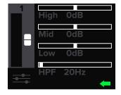
Other than the aforementioned EQ settings screen, this is also where to access the menu screen. From the mixer screen, simply rotate the speaker control knob right until the bottom right icon is illuminated (A). Then push the knob to enter the menu screen (B).
