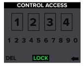
No further changes may be made until the control access is unlocked.
