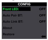
To change a setting, you will just need to rotate the speaker control knob until the configuration you desire to change is illuminated, then push to select it.
