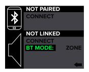
From here, rotate the speaker control knob until the bluetooth mode you prefer is illuminated: zone or stereo. Then push to select.
