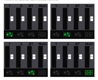
In order to change a channel's EQ, push the speaker control knob when the desired channel's EQ icon is illuminated.
