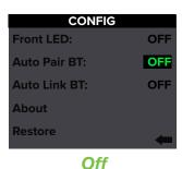
**Auto Link BT** — Allows two previously paired speakers to automatically re-link if both are powered on and in range. When illuminated, push the speaker control knob to select between on or off.
