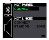
(2) The text "not paired" will change to "discoverable..." and "connect" will change to "cancel". From here, you can either (A) turn the device and device's bluetooth on to pair, or (B) push the speaker control knob to cancel the action.
