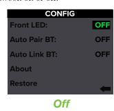
**Auto Pair BT** — Allows a previously paired device to auto reconnect if both the device and speaker are powered on and in range. When illuminated, push the speaker control knob to select between on or off.
