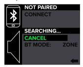
(3) The text "searching..." will change to "primary" on one loudspeaker and "secondary" on the other. Also, "cancel" will change to "disconnect". From here, you can either (A) select a Bluetooth mode (see below), or (B) push the speaker control knob to disconnect.
