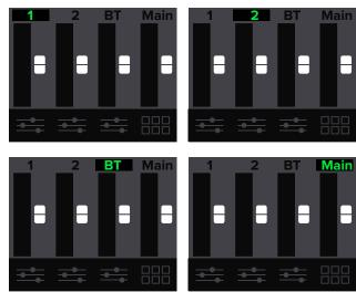
In order to change the level, push the speaker control knob when the desired channel is illuminated. In the same example, notice how the channel 2 fader has been moved to the -5 dB mark. Once the level you desire has been dialed in, press the speaker control knob again to return to the mixer screen.
