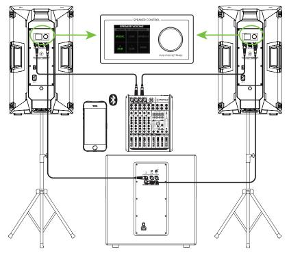
If you desire a little more boom, add a Thump18S subwoofer to the mix. Here, the L/R outputs of a ProFX8v2 mixer are connected directly to the CH1 inputs of each Thump12BST loudspeaker. Then the Mix Out of each loudspeaker is connected to the channel A and B inputs of a single Thump18S subwoofer. Don't forget to set the Speaker Modes to Music + Sub.
