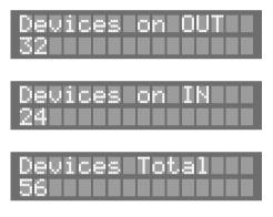
The Device number display shows devices detected on the NomadLink network. Devices are shown for the IN port, the OUT port, and the combined number of devices. The above example shows two singleended daisy-chains connected separately to the IN and OUT ports. However, in most cases a Closed Loop is recommended.
