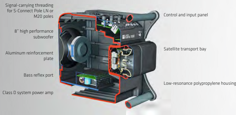
Cross-section of a LUCAS NANO 300 series subwoofer
