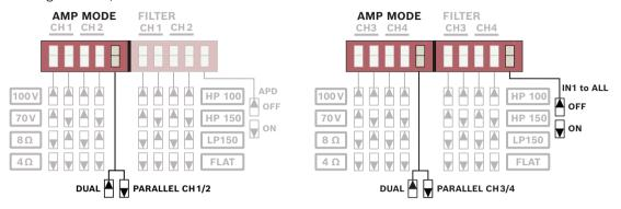
Figure 5.2: Input routing configuration (channel 3 and 4 for V600:4 only)
