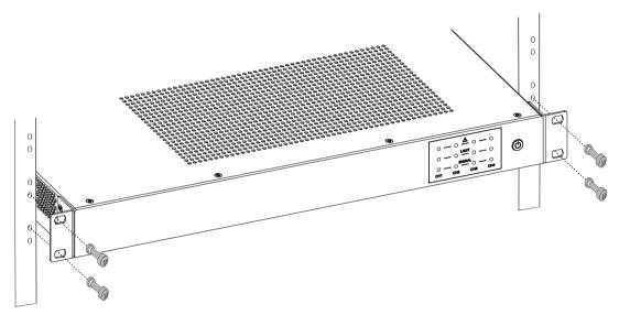
Figure 4.1: Mounting the amplifier in a rack
