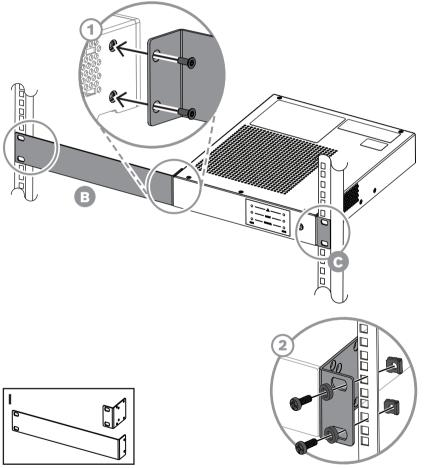
Figure 4.3: Stand-alone mounting in a 19"-rack
