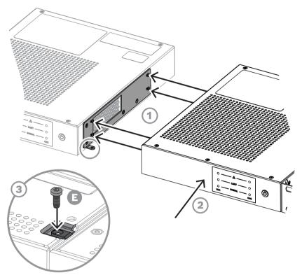
Figure 4.5: Two amplifiers hooked together with connection plate mounted and M3 bolt to prevent
