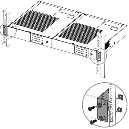
Figure 4.6: Side-by-side mounting in a 19"-rack
