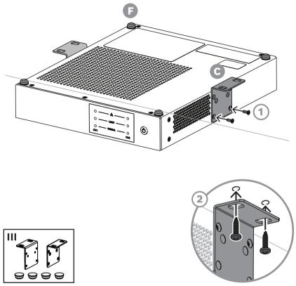
Figure 4.7: Tabletop use - under the table
