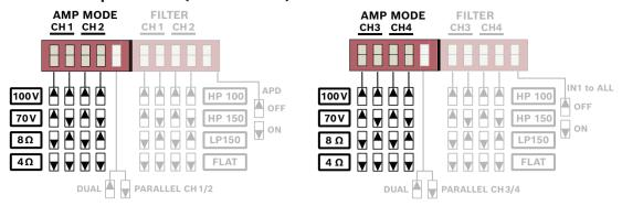
Figure 5.1: Output mode configuration (channel 3 and 4 for V600:4 only)
