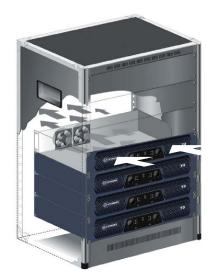
Figure 2: Proper rack venting
