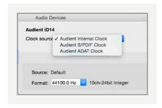
If you are using Windows, go to the iD icon in the system tray and right click on it. This will bring up some settings including sample rate. Alternatively you can alter these settings in the Setup tab of the iD app.
