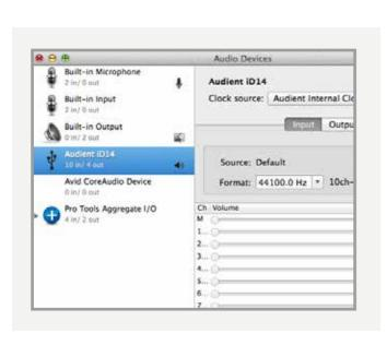
Double check that an appropriate clock source is selected (Internal for master operation), ADAT or S/PDIF clock for external slave operation. Ensure that you see the correct sample rate displayed in the Format drop-down menu.
