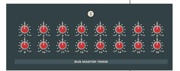
BUS MASTER TRIM controls the overall level of a bus output.
